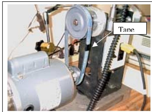
Think about what this is going to do. Once per revolution of the belt, this lump is going to go over the driven sheave (and the driver but we aren't measuring the driver.) The rise of the belt is going to increase belt tension and put a hard downward force on the driven sheave. We would expect, then, to find vibration frequency at 1X the belt pass frequency.
